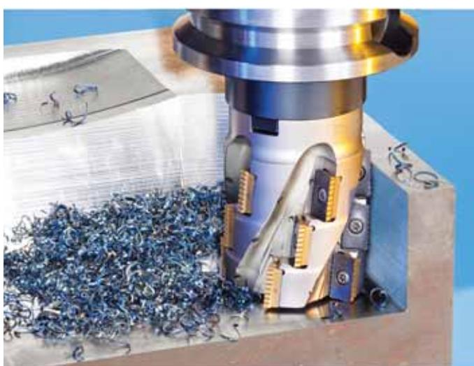
Obr. 2 Fréza MILLSHRED
